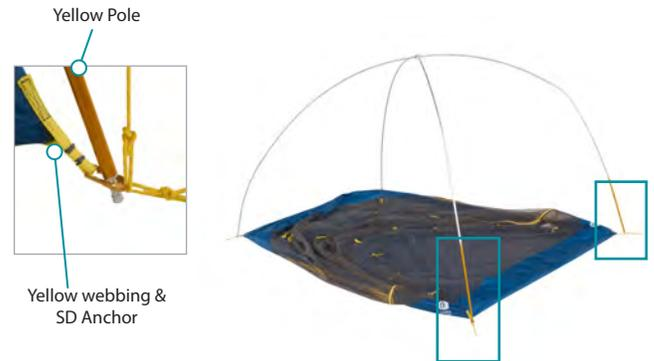
**STEP 3:** Connect Tent Lite hooks to poles. Attached yellow ridge pole to Ball Cap Connectors.
